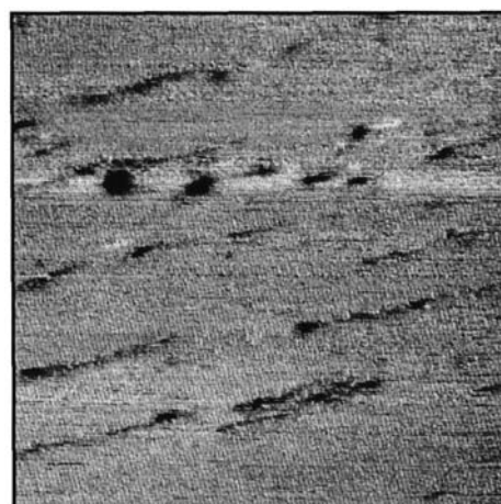
Figure 3. Well-ordered and close-packed structure of 3-octylthiophene SAMs on Au(111): 53 \times 53 \text{ nm}^2 , I_t = 0.15 \text{ nA} , and V_b = 0.41 \text{ V} (sample positive).
